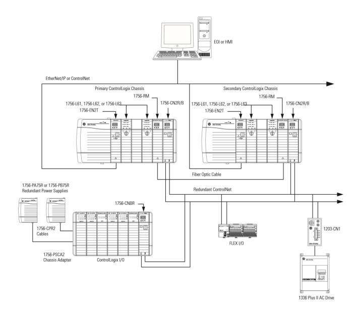
modules to span many applications, from high-speed digital to process control. The ControlLogix architecture uses Producer-Consumer technology, which allows input information and output status to be shared among multiple ControlLogix controllers.
