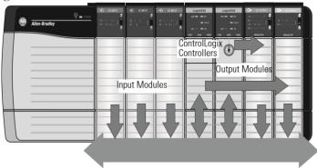
Each ControlLogix I/O module mounts in a ControlLogix chassis and **requires** either a removable terminal block (RTB) or a 1492 interface module (IFM) to connect all field-side wiring. RTBs and IFMs are not included with the I/O modules. They must be ordered separately.
