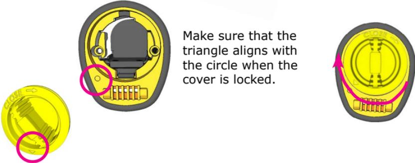
Make sure that the triangle aligns with the circle when the cover is locked.
