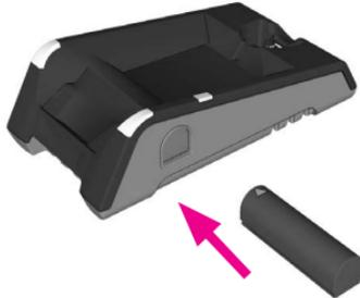
When you are charging the auxilliary battery, the base station's spare battery status indicator displays either charging in progress (red) or fully charged (green).
