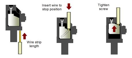
Figure 426: Wire Preparation and Insertion into Box-Style Terminal Block
