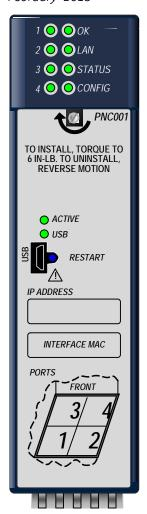
The PACSystems\* RX3i PROFINET Controller (PNC) module, IC695PNC001, connects a PACSystems RX3i controller to a high-speed PROFINET local area network. It enables the RX3i controller to communicate with I/O-Devices on the LAN. The PNC provides all the functions, services, and protocols required for certification as a PROFINET I/O Version 2.2 I/O Controller, running at both 100 Mbps and 1 Gbps.
