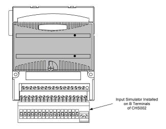
The Input Simulator can be installed in either the A or B terminals of the carrier, depending on which module inputs should be controlled. After inserting the pins of the Input Simulator, tighten down the screws on the carrier.
