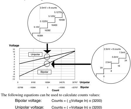
For a change in the reported count value to be seen, input current must be increased by at least 2.5mV. If the module receives an increase less than 2.5mV, the previous count value is still reported. For example:
