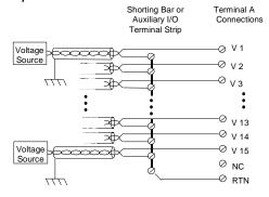
An optional Shorting Bar or Auxiliary I/O Terminal Strip can be used for wiring convenience, when multiple return paths need to be wired together.
