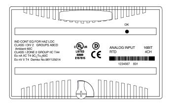
No external power supply is required for this module. The excitation current for the RTDs is provided by the module, which automatically matches the excitation current to each configured RTD type.
