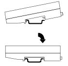
All connecting carriers must be installed on the same section of 35mm x 7.5mm DIN rail. The rail must have a conductive (unpainted) finish for proper grounding. For best stability, the DIN rail should be installed on a panel using screws spaced approximately 6 inches (5.24cm) apart.
