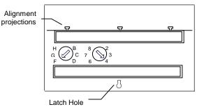
Press the module straight down onto the carrier, seating it fully.
