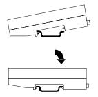
All connecting carriers must be installed on the same section of 35mm x 7.5mm DIN rail. The rail must have a conductive (unpainted) finish for proper grounding. For best stability, the DIN rail should be installed on a panel using screws spaced approximately 6 inches (5.24cm) apart.
