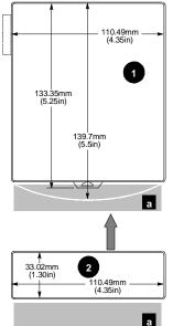
Carriers must be mounted on a horizontal DIN rail.
