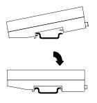
The CPU and connecting carriers must be installed on the same section of 35mm x 7.5mm DIN rail, 1mm thick. Steel DIN rail is recommended. The DIN rail must be electrically grounded to provide EMC protection. The rail must have a conductive (unpainted) corrosion-resistant finish. DIN rails compliant with DIN EN50032 are preferred.
