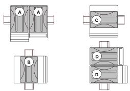
For IC200MDL243 and BXIOIAI16120 modules that are mounted horizontally (C, D) on the DIN rail, no derating is required at 120VAC. Deratings at 132VAC are shown below.
