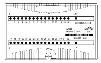
Power for module operation comes from the backplane. Intelligent processing for the module is performed by the CPU or NIU.
