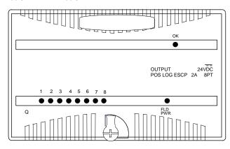
An external DC power supply must be provided to switch power to the loads.
