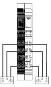
The sensors are powered by a Segment Terminal module (left). They can also be supplied from an external power supply.
