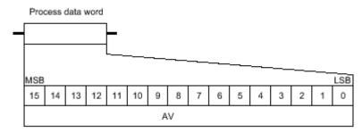
The process data output word specifies the output value in each cycle. All output values have 16 bit resolution.
