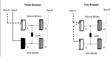
If the blocks are on three busses, one source and one sink block in the group must be on the same bus. The two blocks on the same bus must have different serial bus addresses. If the blocks are on two busses, one source and one sink block are on one bus and the other source and sink block are on the other bus. Any blocks that share a bus must have different serial bus addresses.
