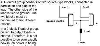
16-circuit blocks in a 2-block T output group are configured for No Load fault reporting, the minimum connected load that can be used is 100mA.
