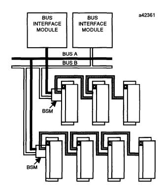
The locations of BSMs depend on the type of bus trunk cable and baud rate, as explained below.
