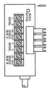
A phase B discrete block in the cluster controls the operation of the Bus Switching Module. The first circuit on this discrete block functions as an output dedicated to the BSM. This output causes the BSM to switch busses if communications are lost on the current bus.
