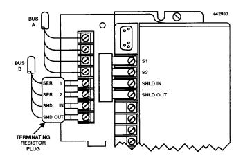
If both cables terminate at the BSM, install two resistors.
