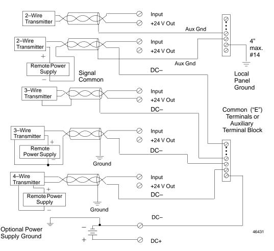
I/OTerminal Block wiring assignments for this module are shown below.
