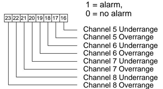
**Channel Under/Overrange Bits (byte 1)**
