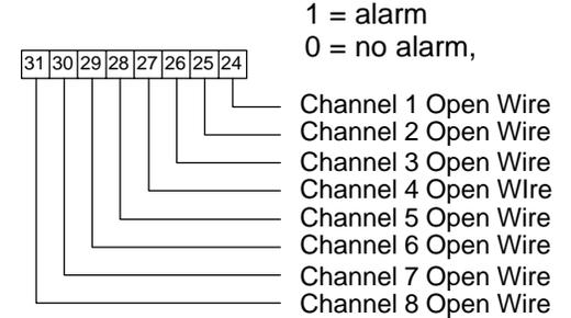
**8 Point Analog Current-Source Output Module****Clearing Faults and Alarms**
