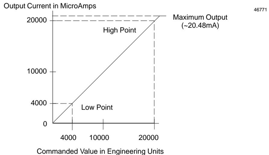
Scaling can be customized by changing any of the engineering units and/or output current values for each point. Span (output current) values are unsigned integers ranging from 0 to 20,000. Engineering units values are 16-bit signed integers from -32,768 to 32,767.
