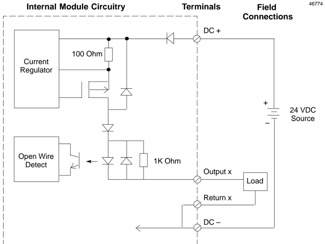
The 8 Point Analog Current-source Output Module provides the following alarms:
