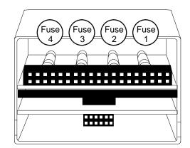
Carefully pry the fuse upward to remove it, taking care not to damage any components in the module. Place the new fuse in position and press it into the holder.
