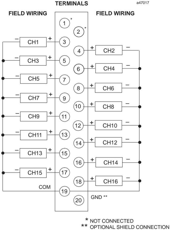
**Figure 10-11. Field Wiring for 16-Channel Analog Voltage Input Module - IC693ALG222 (Single-Ended Mode)**
