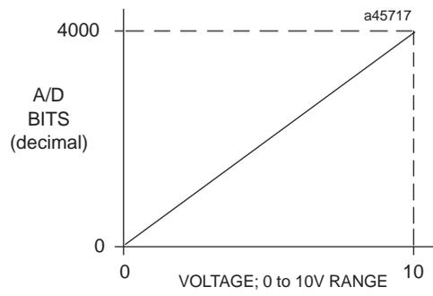
**Figure 10-10. A/D Bits vs. Voltage Input for IC693ALG222**
