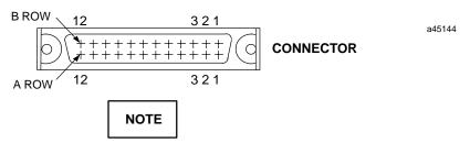
Each wire pair has a solid color wire and that same color wire with a black tracer. For example, Pair 1 has a solid brown wire paired with a brown wire with a black tracer.
