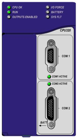
The PACSystems\* RX3i CPU can be used to perform real time control of machines, processes, and material handling systems. The CPU communicates with the programmer and HMI devices via a serial port using SNP Slave protocol. It communicates with I/O and smart option modules over a dual backplane bus that provides:
