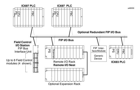
Figure 1. Example of FIP Bus Controller In a System
