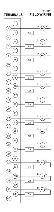
**Figure 2. Field Wiring Connections**
