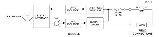
Figure 1. Block Diagram for IC697MDL341
