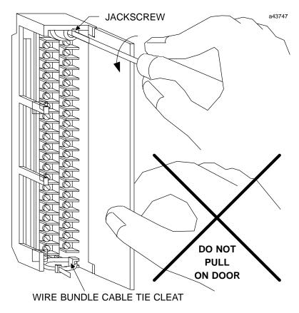
Figure 4. Removal of I/O Terminal Board
