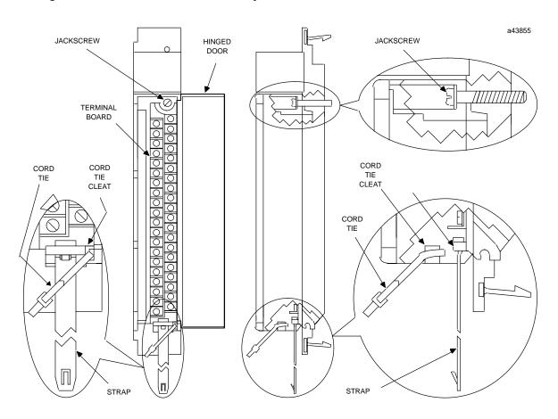
Figure 3. I/O Module Features
