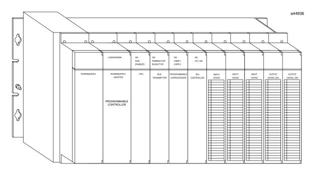
Figure 1. Location of Power Supply Adapter Module in an IC697 PLC Installation
