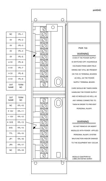
It is recommended that the external power supply have a +5V Remote Sense. When the Remote Sense is connected to the PSA terminal board (positive remote sense to +5VS and negative to 0VS) the +5 volts at the backplane will be regulated to the level set by the power supply.
