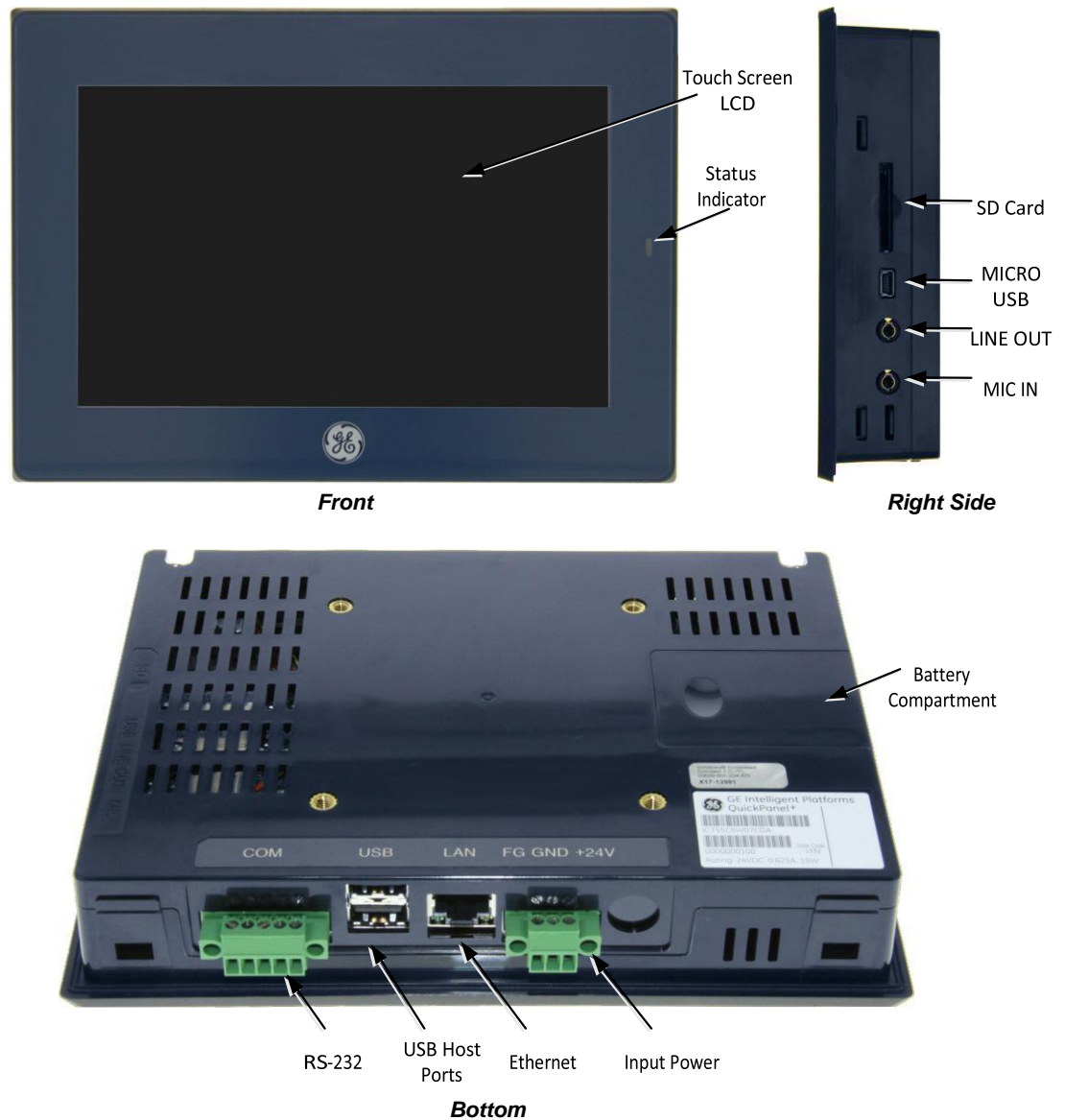
Figure 1. QuickPanel+ Hardware Features
