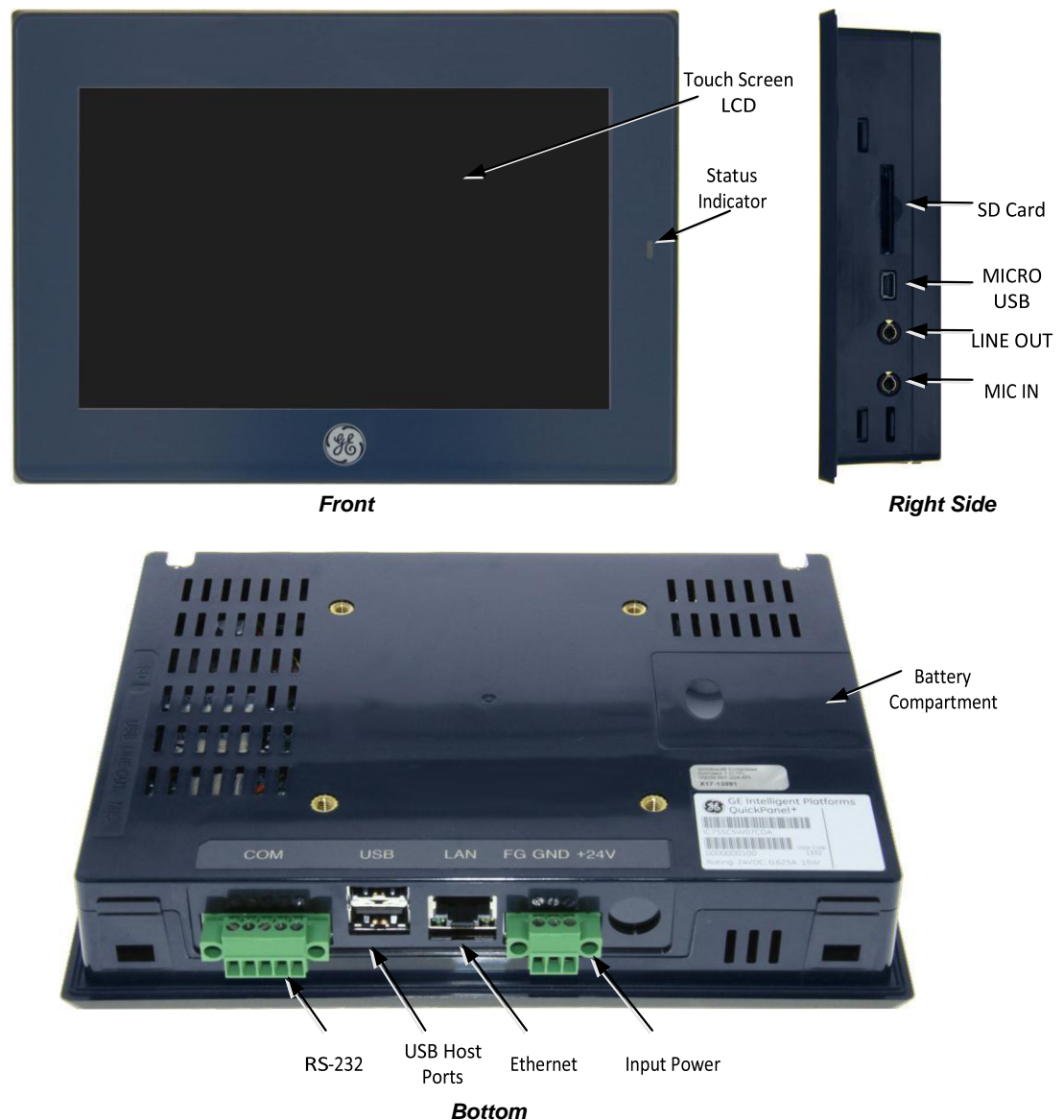
Figure 1. QuickPanel+ Hardware Features
