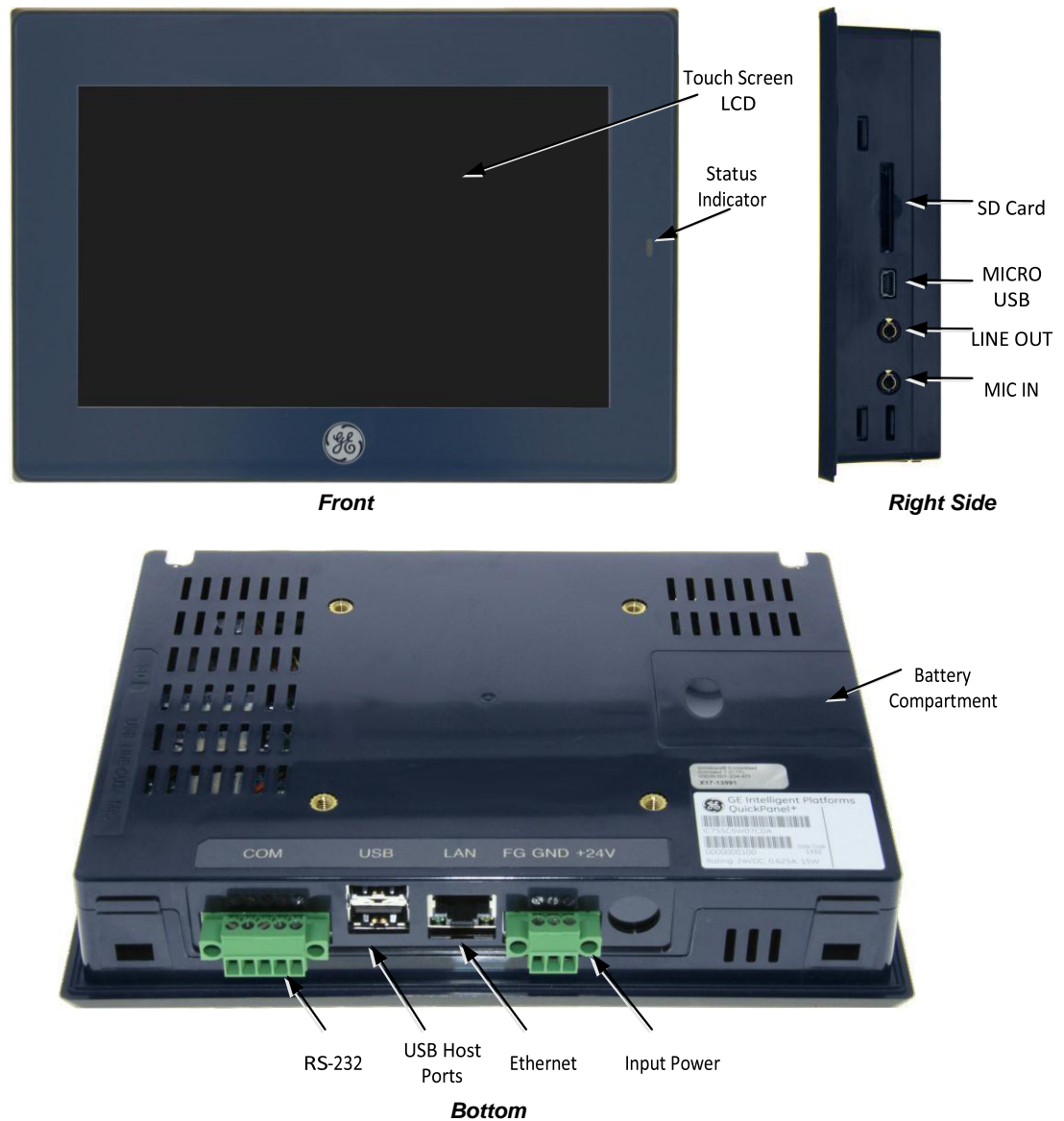
Figure 1. QuickPanel+ Hardware Features
