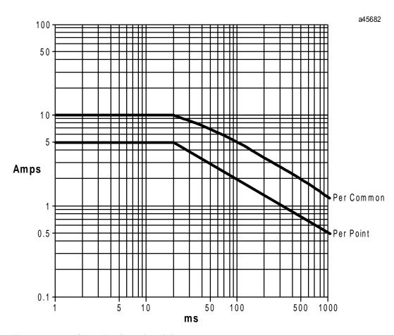
Figure 4-11. Inrush Derating Curve for AC Output
