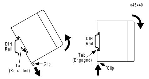
Position the upper edge of the unit over the DIN rail, so that the rail is behind the tab as shown above. Pull the clip down. Pivot the unit downward (for a unit being mounted right side up) until the unit is over the DIN rail. Press the clip firmly into place.
