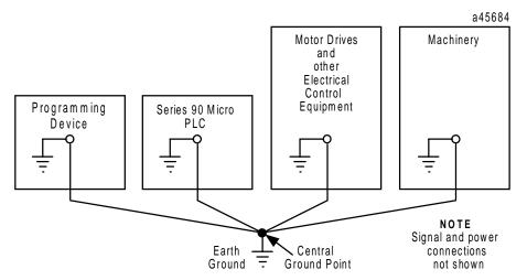
Figure 3-4. Recommended System Grounding
