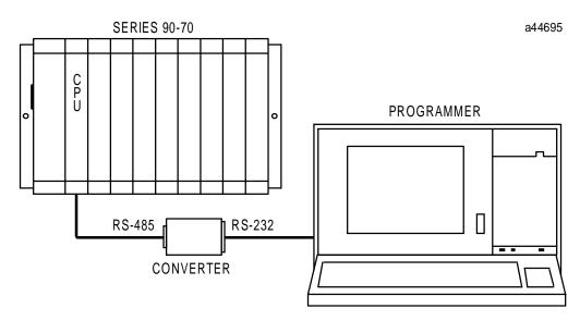
Figure E-2. Typical Configuration with Series 90-70 PLC
