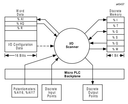
Figure 8-4. Series 90 Micro PLC I/O Structure
