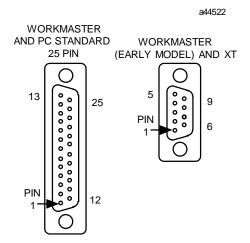
Figure D-2. Workmaster RS-232 Serial Port Connector Configuration
