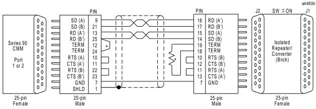
\* Terminate connection: On the CMM, Install jumper to connect internal 120 ohm resistor. On the isolated repeater/converter, install 150 ohm resistor (supplied).
