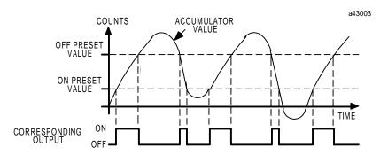
If the output is enabled for the HSC channel being used, the output will turn on in accordance with the following table:
