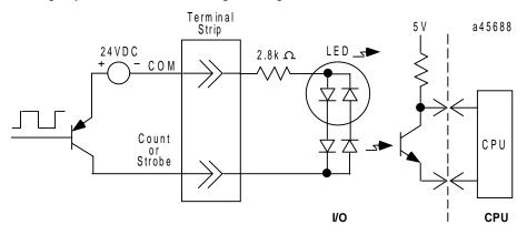
Figure 4-3. High Speed Counter Circuit - Positive Logic Connection
