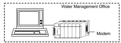
The master Series 90-30 PLC collects data from the remote Series 90 Micro PLCs and sends it to the CIMPLICITY system, which has overriding control of the system.
