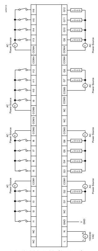
Figure 4-15. 28-Point AC In/AC Out Modules (IC693UAA007)
