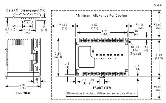
Figure 3-2. Micro PLC Mounting Dimensions and Spacing Requirements, 14-Point
