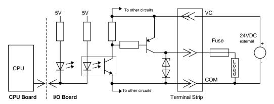
Figure 4-6. Typical Transistor Output Circuit 24 VDC
