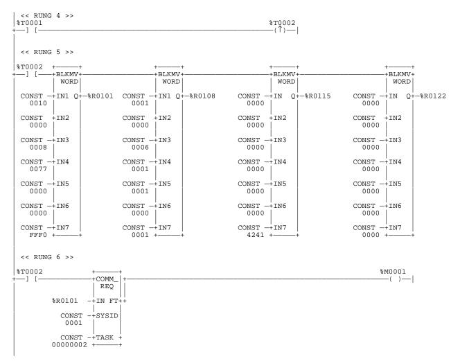
Figure 5-1. Ladder Logic Example for Serial Port Configuration
