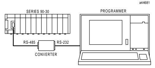
Figure E-3. Typical Configuration with Series 90-30 PLC
