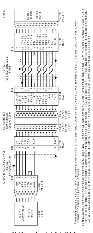
Figure D-5. IBM-AT (compatibles) Personal Computer to Series 90 PLCs
