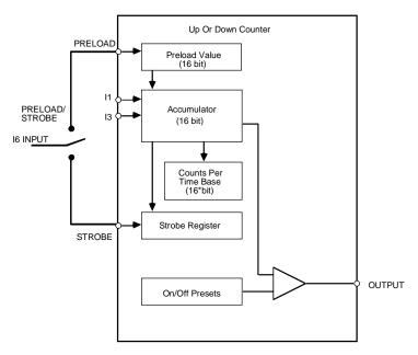
Figure 6-2. Type B Counter Block Diagram
