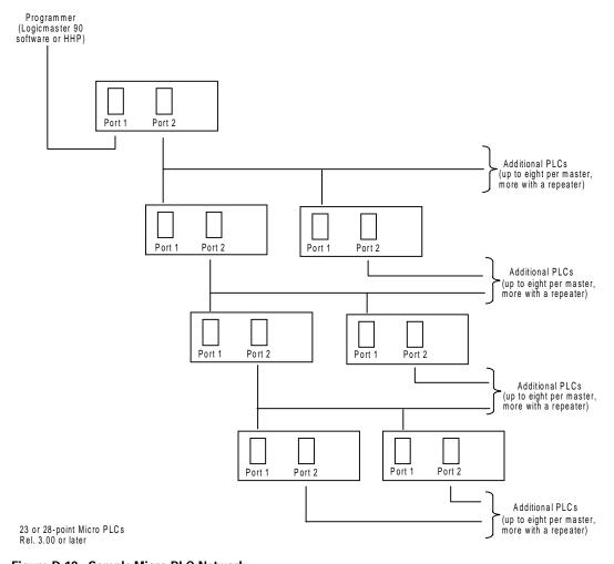
Figure D-19. Sample Micro PLC Network
