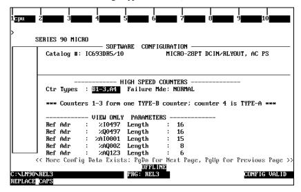
The following screen presents the configuration parameters for the type B counter. (On DC-output Micro PLCs, Pulse and PWM outputs are not available when the type B counter is configured.) Refer to Table 6-6 for parameter definitions. For details on how these parameters control operation of B-type counters, refer to page 6-16.
