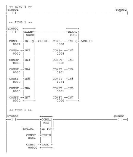
Figure 6-3. Ladder Logic Example for Setting a High Speed Counter Parameter
