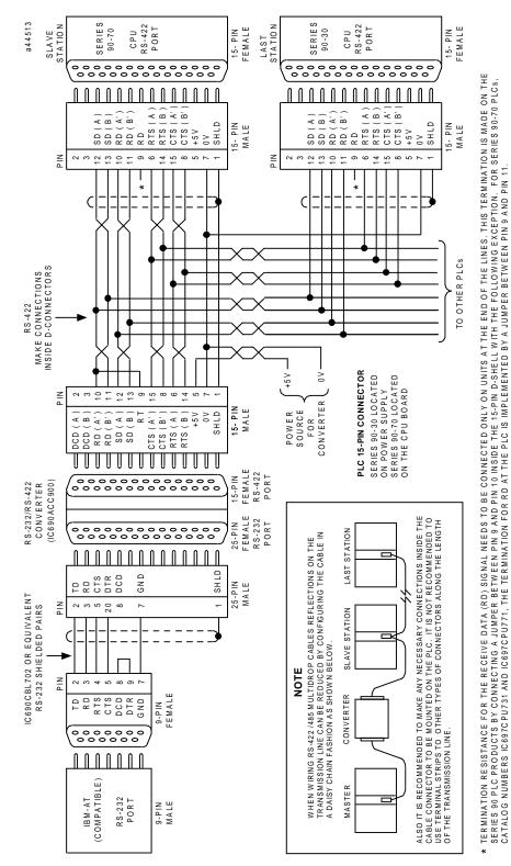
Figure D-11. IBM-AT/Series 90 PLC Multidrop Connection
