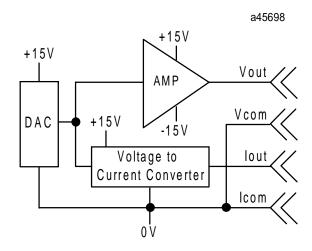
Figure 4-8. Analog Output Circuit
