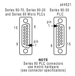
Figure D-1. Series 90 PLC, RS-422 Serial Port Connector Configuration
