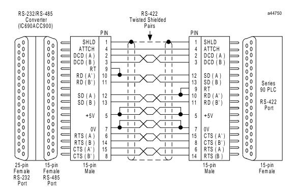
Note: Plns 9 and 10 are jumpered at both ends of cable to connect terminating resistors for the RD signal which is inside the PLC power supply.
