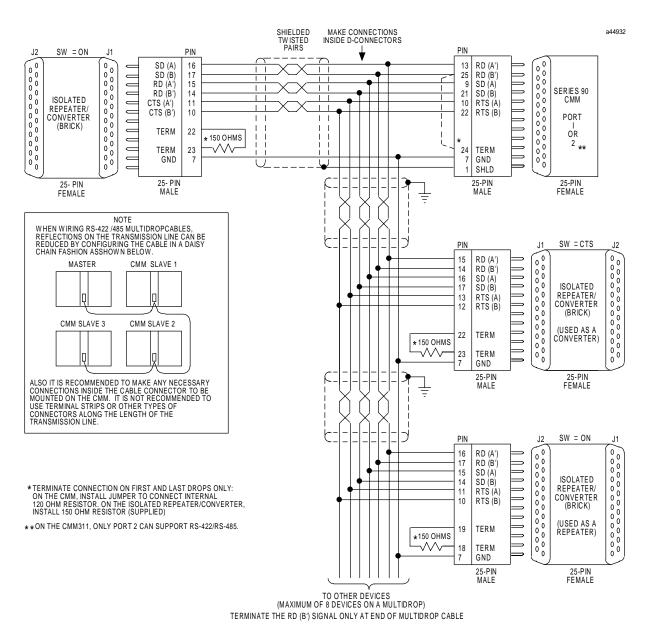
Figure E-18. Cable D: RS-422 Twisted Pair
