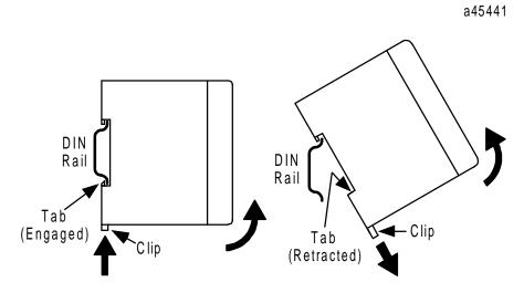
Pull clip at the bottom of the unit down until it is disengaged from the DIN rail.
