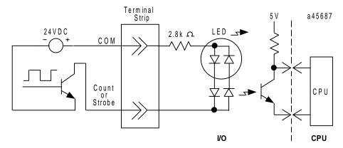
Figure 4-2. High Speed Counter Circuit - Negative Logic Connection
