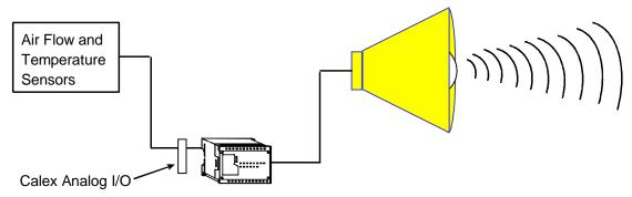
The Series 90 Micro performs logic on input from the sensors to alert the town of pending tornadoes and other forms of severe weather.
