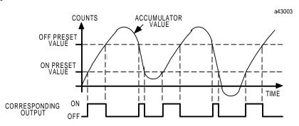
If the output is enabled for the HSC channel being used, the output will turn on in accordance with the following table:
