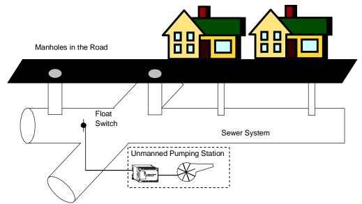
Series 90 Micro PLCs use float switches to monitor the level of water in the sewer system. During storms it cycles relief pumps on and off to prevent the backup of water into houses and businesses.
