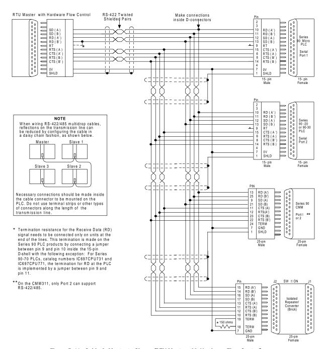
Figure D-16. Cable A: Master to Slaves (RTU Master with Hardware Flow Control)
