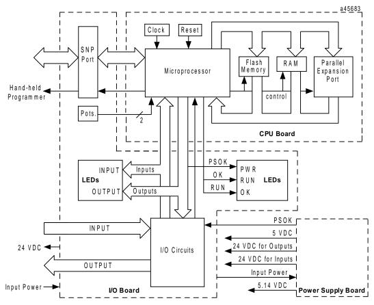
Figure 2-2. Micro PLC Functional Block Diagram
