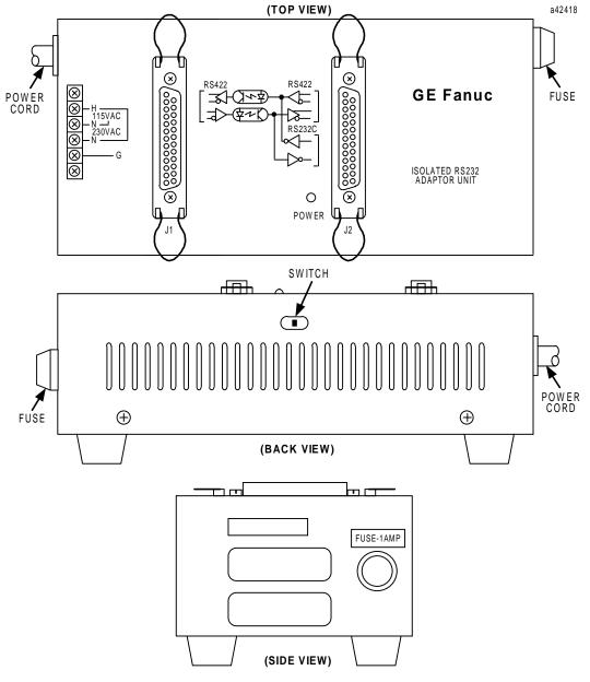
Figure E-10. Isolated/Repeater Converter
