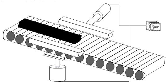
The Series 90 Micro PLC receives input from photo sensors on the conveyor to control the cylinders that position the boards.
