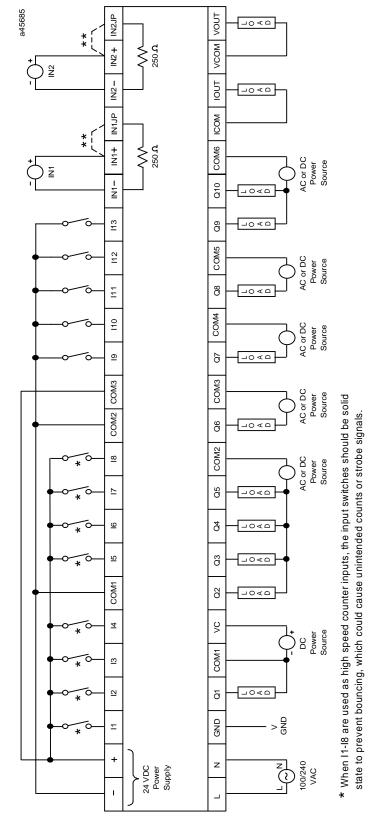
Figure 4-16. 23-Point DC In/Relay and DC Out (IC693UAL006)
