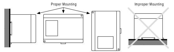
Figure 3-1. Recommended Mounting Orientations for the Micro PLC
