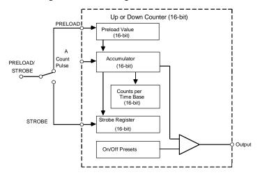
Figure 6-1. Type A Counter Block Diagram
