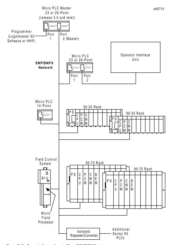
Figure D-13. Example Connections to Micro SNP/SNPX Master
