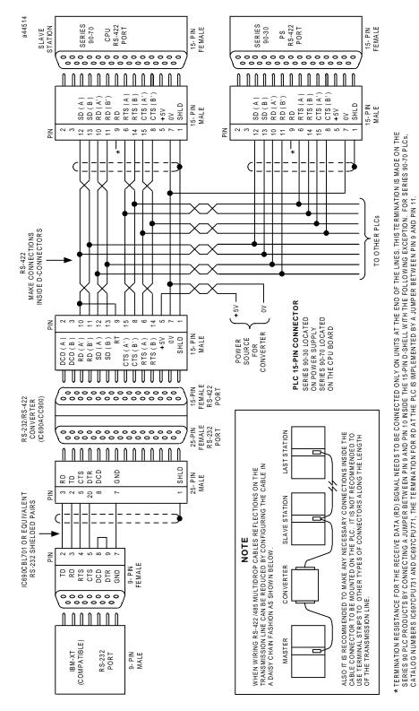
Figure D-12. IBM-XT/Series 90 PLC Multidrop Connection
