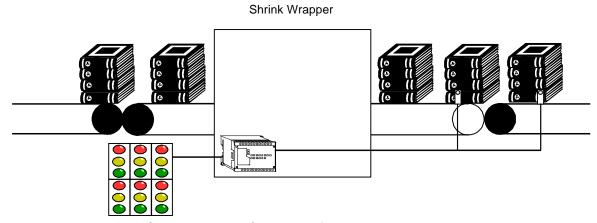
The Series 90 Micro PLC uses input from various sensors to determine the position of product and parameters from the control panel to sequence the wrapping of the products.
