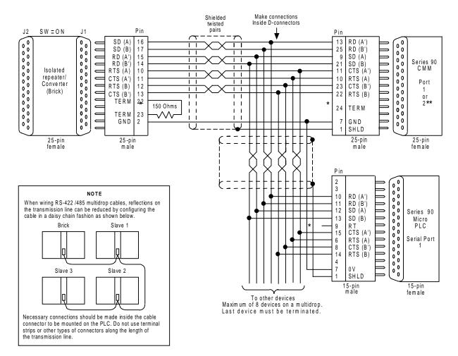
\* Termination resistance for the Receive Data (RD) signal needs to be connected only on units at the end of the lines. This termination is made on the Series 90 PLC products by connecting a jumper between pin 9 and pin 10 inside the 15-pin D-shell with the following exception: For Series 90-70 PLCs, catalog numbers IC697CPU731 and IC697CPU771, the termination for RD at the PLC is implemented by a jumper between pin 9 and pin 11.
