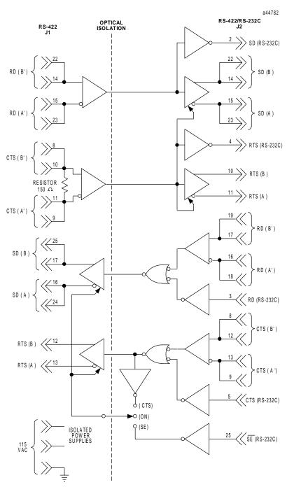
Figure E-11. RS-422 Isolated Repeater/RS-232 Converter Logic Diagram
