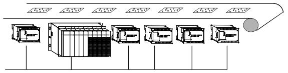
Series 90 Micro PLCs control individual sections of the conveyor as the Series 90-70 PLC controls the overall system.
