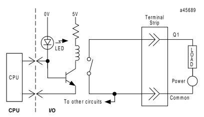
Figure 4-4. Typical Relay Output Circuit
