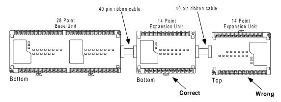
Figure 3-11. Micro Expansion Unit Orientation
