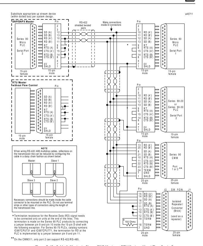
Figure D-15. Cable A: Master to Slaves (SNP Master or RTU Master without Flow Control)
