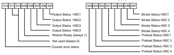
**Strobe/Preload Status:** The HSC sets these bits when a strobe or preload occurs. The CPU must clear the bit using the corresponding Reset Strobe/Reset Preload output.
