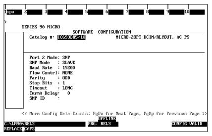
Table 5-3. Configuration Parameters for Serial Port 2
