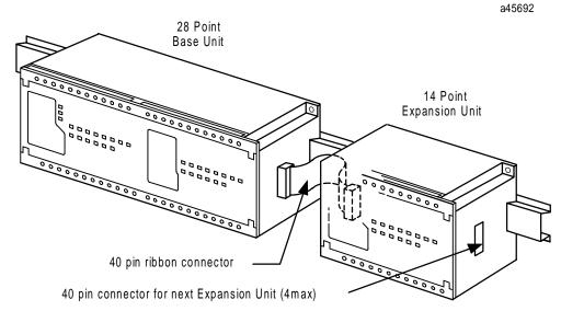
Figure 3-10. Expansion Unit Installation
