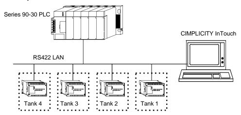
Each Series 90 Micro PLC controls a tank and is also connected to the master Series 90-30 PLC for override control.
