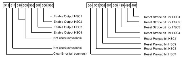
**Enable Output** Bits 505 through 508 are used to enable or disable the module's outputs. If an
