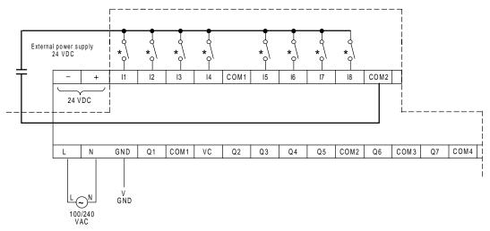
\* High speed counter inputs should be powerd separetly from discrete inputs. The switching devices should be solid state to avoid bounce, which could cause unintended counts or strobes.
