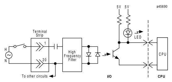
Figure 4-9. Typical 120 VAC Input Circuit
