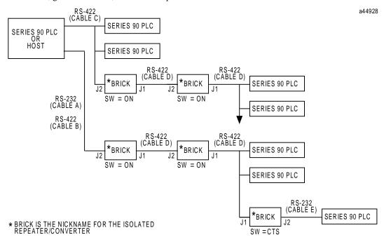
Figure E-14. Complex System Configuration Using the Isolated Repeater/Converter
