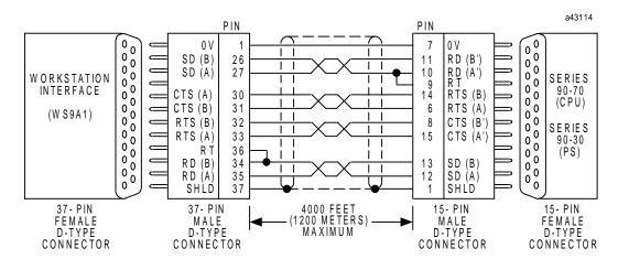
Figure F-4. Series 90 PLC to Workmaster II Serial Cable
