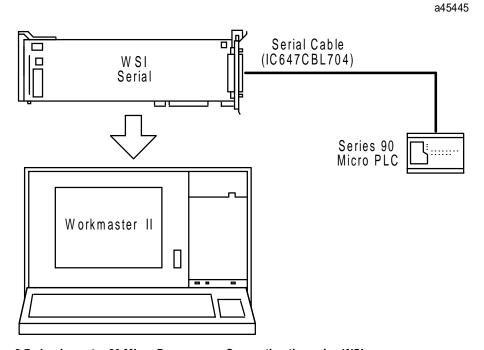
Figure 3-7. Logicmaster 90 Micro Programmer Connection through a WSI
