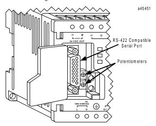
Figure 2-3. Micro PLC RS-422 Serial Port
