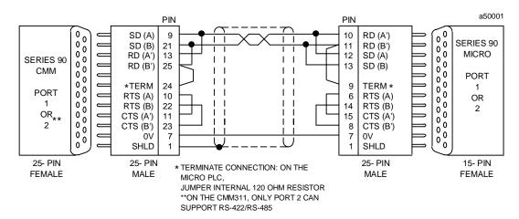
Figure F-6. CMM to Micro with Flow Control=None (2-Wire RS-422/RS-485)
