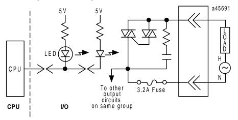
Figure 4-10. Typical 120 VAC Triac Output Circuit
