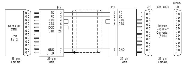
Figure E-15. Cable A: RS-232 CMM To Converter
