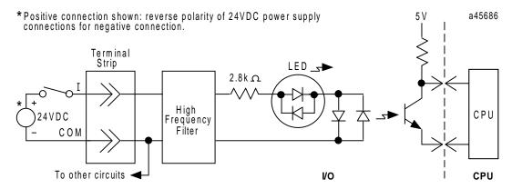
Figure 4-1. Typical 24 VDC Positive/Negative Logic Input Circuit
