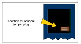
In a non-redundancy application, where automatic restarting may be appropriate, a shunt can be installed on back of the module as shown at left. The shunt must have 0.100 inch spacing on center and accommodate 0.025 inch pins. Example parts are Radio Shack DIP Programming Shunt #276-1512 and DIGI-Key #59000-ND. The module must be removed from the backplane to install the shunt.
