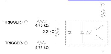
28VDC Max. Across input pins - Transition approx. 8VDC (Nom.)
