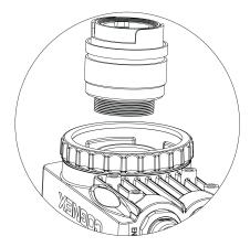
3. If using a lens cover, remove the thread guard and attach the lens to the vision system.
