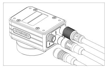
5. Restore power to the 24VDC power supply and turn it on if necessary.
