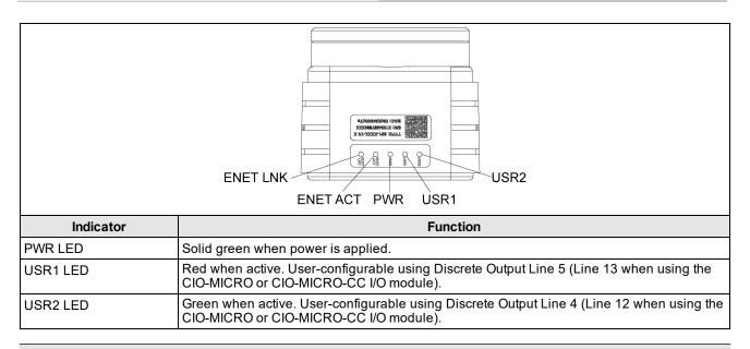
Note: If the USR2 LED blinks green three times followed by the USR1 LED blinking red sixteen times, the vision system is not operating correctly. If power cycling does not resolve the problem, please contact Cognex Technical Support.
