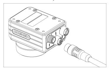
3. Connect the other end of the Light cable to an external lighting device (for example, a strobe light). For more information, refer to the *Light Cable Specifications* on page 29.
