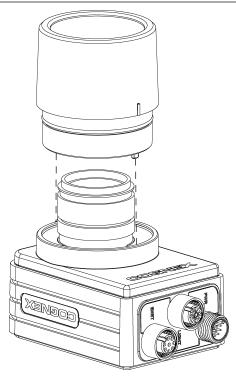
b. Turn the lens cover clockwise until it is in the locked position.
