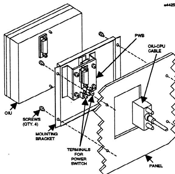
Figure 3-23. Installing the OIU Mounting Bracket
