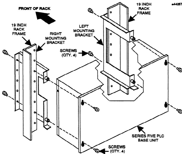
**Figure 3-2. Base Unit Installation in a 19 Inch Rack**
