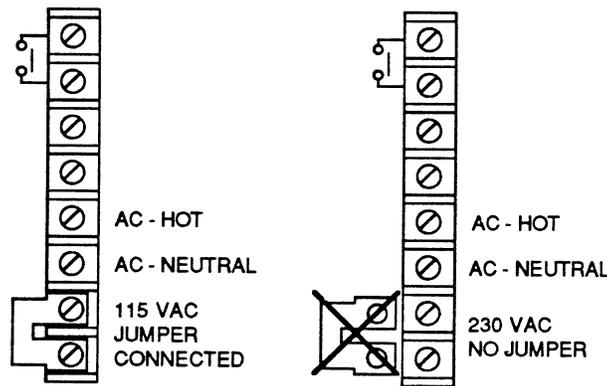
**Figure 2-13. Configuration of Terminal Jumper for 115 or 230 V AC Power**
