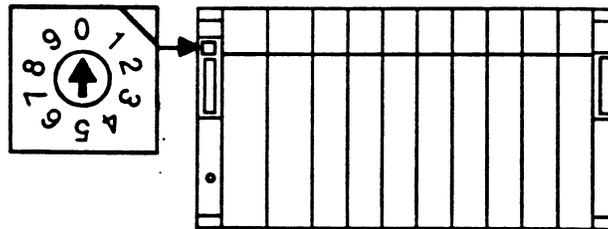
Figure 3-5. Base Unit Identification Selection
