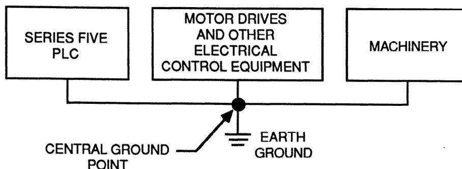
**Figure 3-9. Recommended PLC System Grounding**
