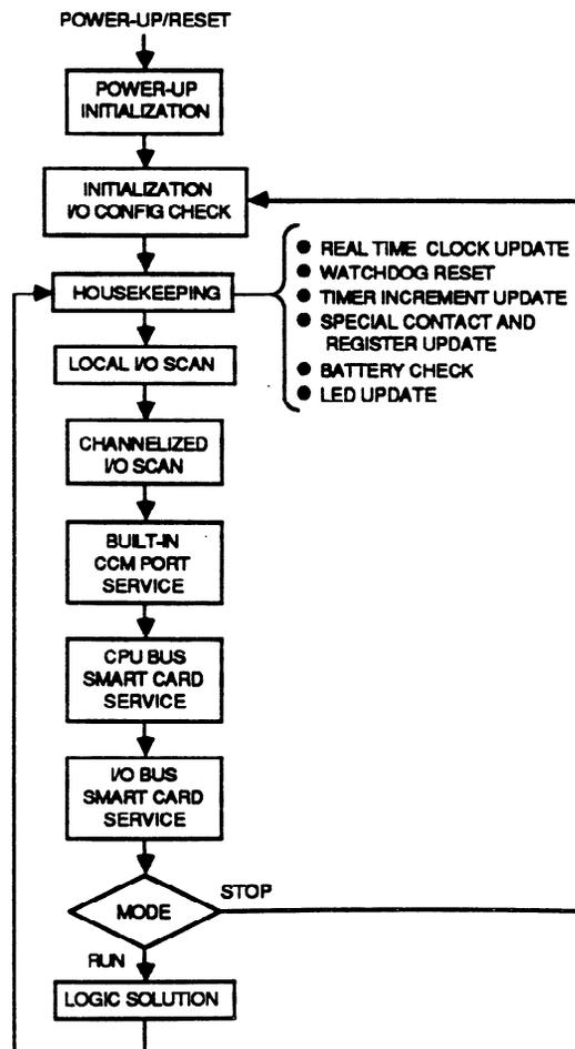
Figure 1-7. Series Five CPU Scanning Sequence
