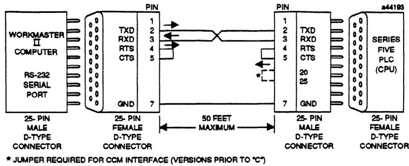
Figure 2-30. Series Five PLC Serial Port to Workmaster II
