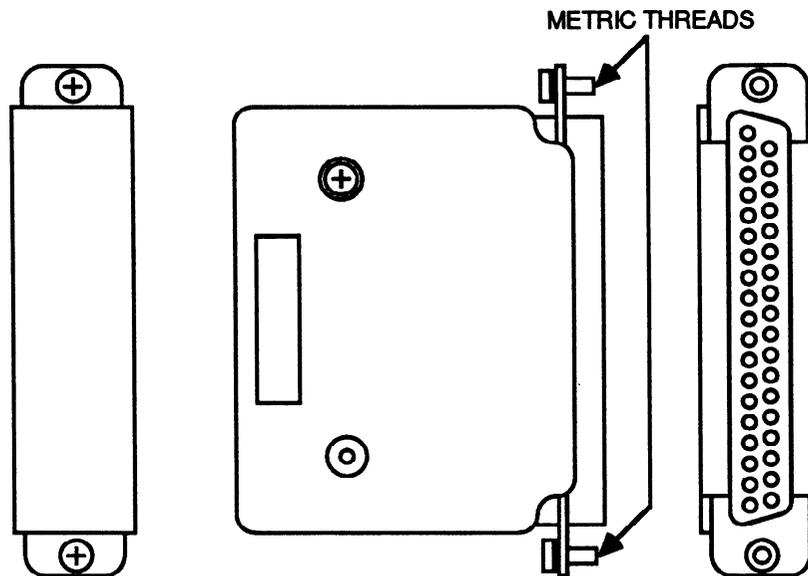
Figure 2-20. I/O Chain Terminator Plug
