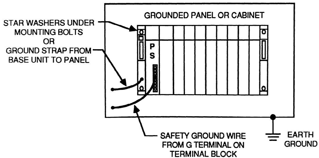
**Figure 3-10. Base Unit Safety and Signal Ground Connections**
