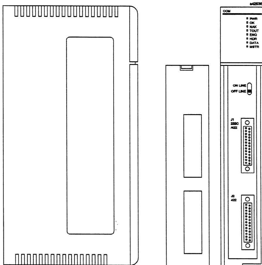
Figure 2-25. Series Five PLC CCM Communications Module
