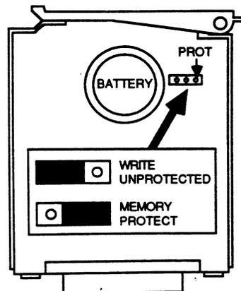
**Figure 3-14. Jumper Positions for Memory Protect Configuration**
