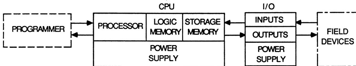
**Figure 1-1. Programmable Logic Controller Block Diagram**
