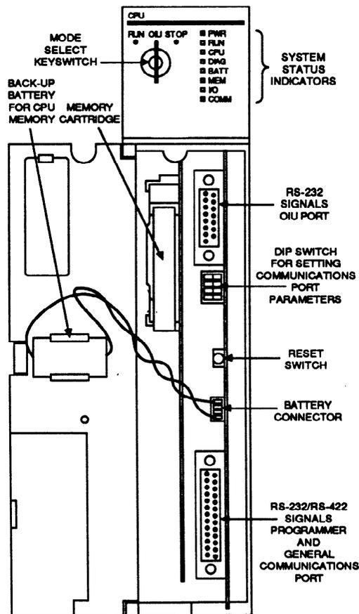
Figure 2-3. Series Five CPU Module
