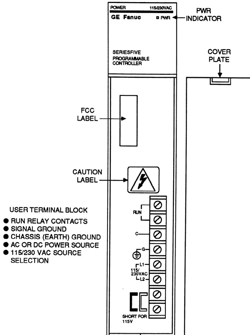
Figure 2-11. Series Five PLC Power Supply
