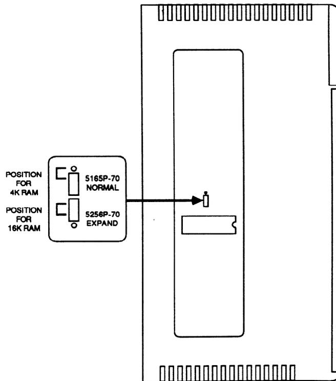
Figure 2-10. 4K/16K Register Jumper Configuration
