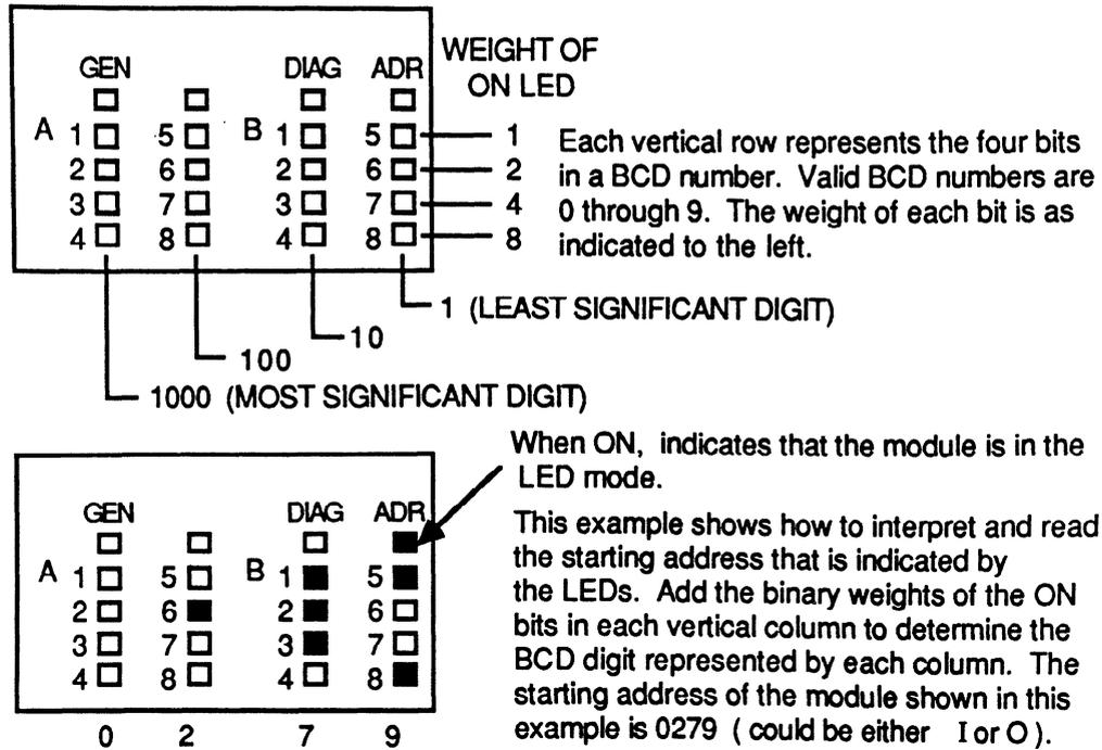
Figure 4-4. Reading I/O Module Starting Address on LEDs
