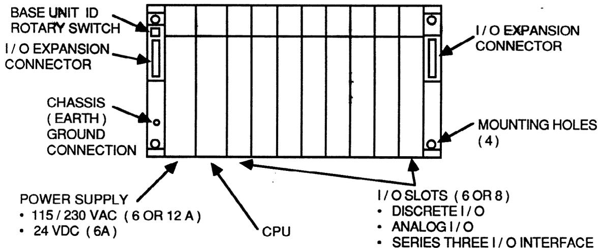
**Figure 2-1. Basic Product Structure for the Series Five PLC**
