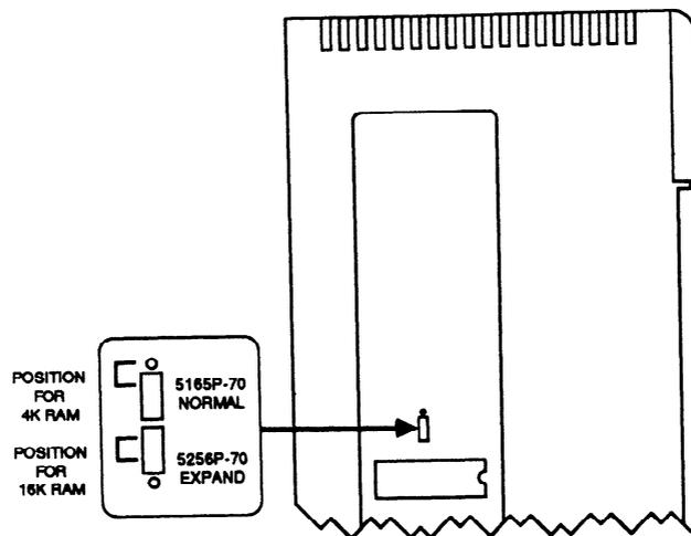
**Figure 3-15. Socket for Register Memory Expansion**
