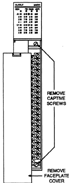
**Figure 5-5. Removal of Terminal Block From Module**
