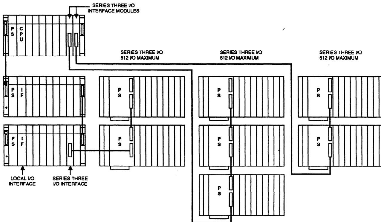
Figure 3-21. Example of Series Five PLC System Using Series Three PLC I/O
