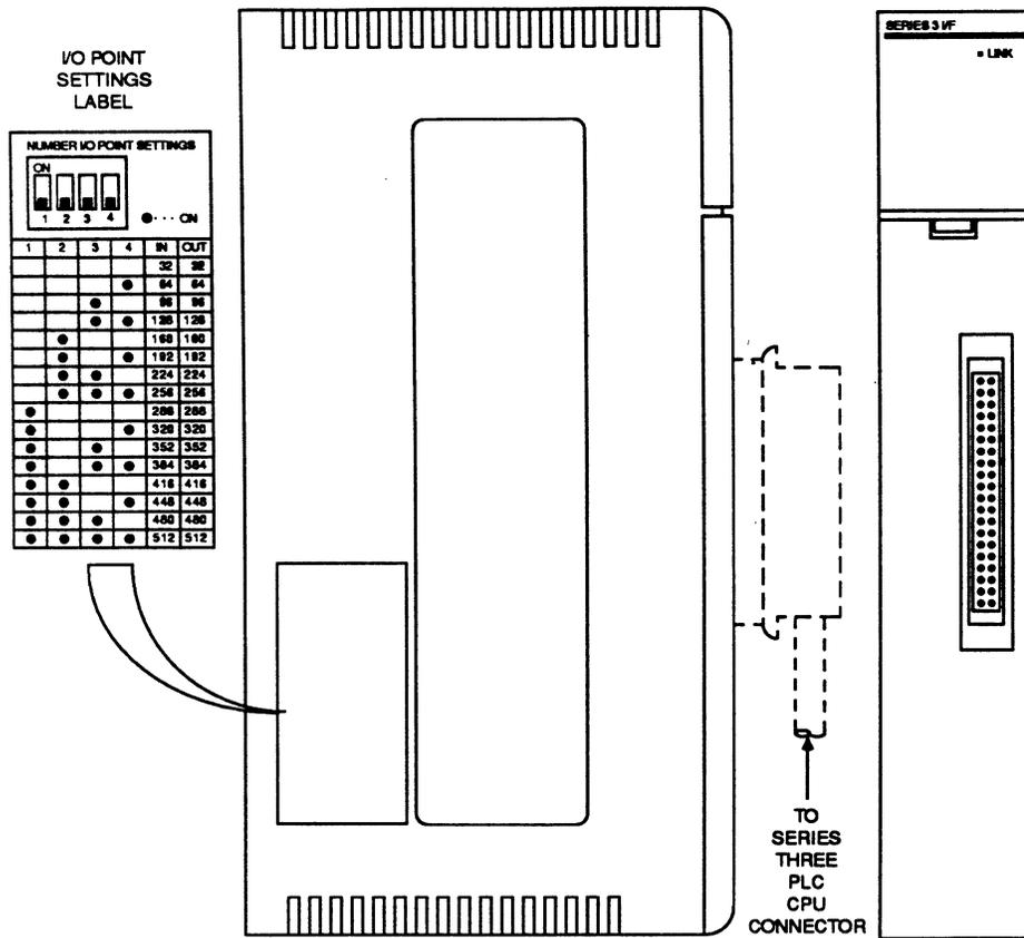
Figure 2-23. Series Three PLC I/O Interface Module
