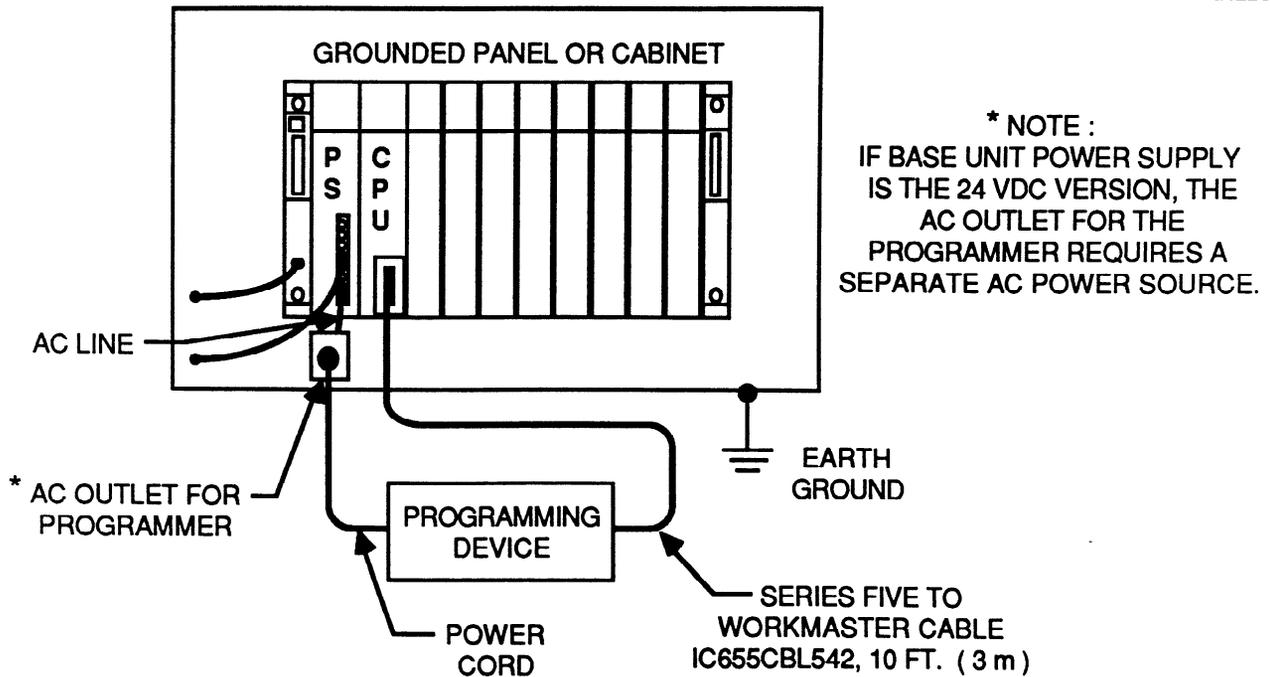
**Figure 3-11. Programming Device Ground Connection**
