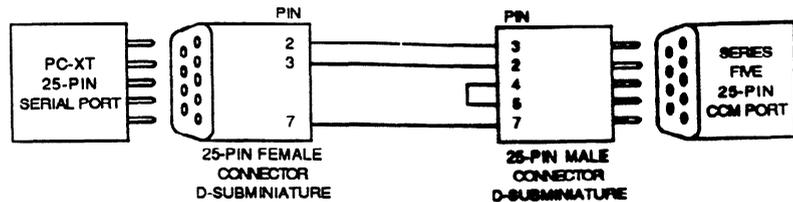
Figure 2-32. Cable for Series Five to PC-XT Computer
