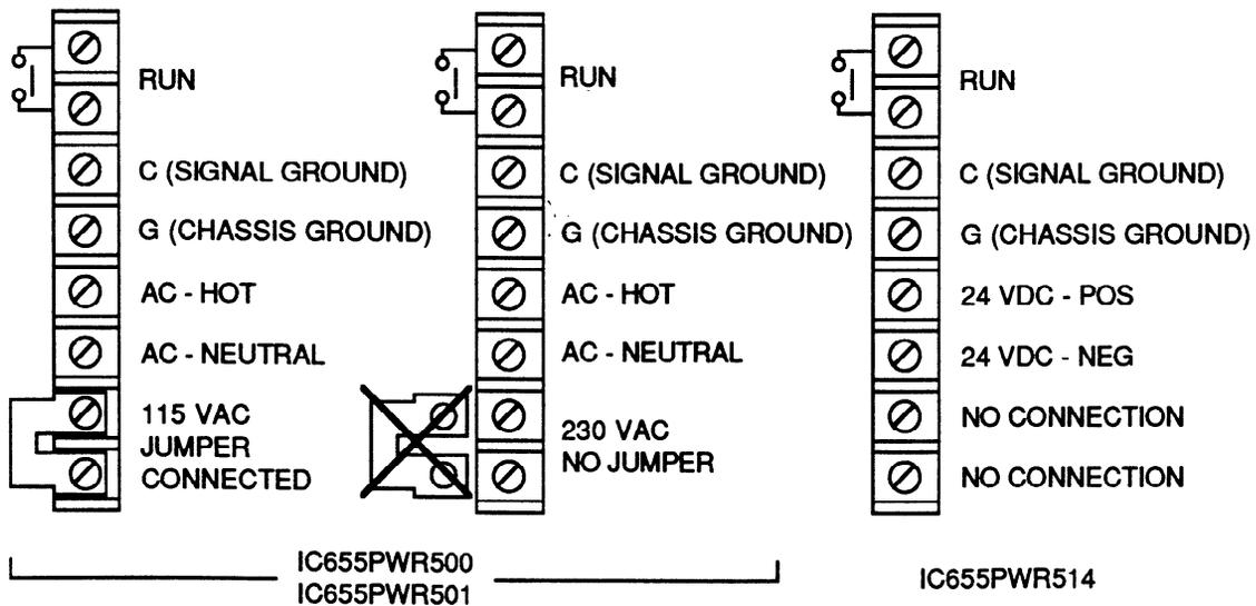
Figure 5-2. Power Supply Terminal Block Connections
