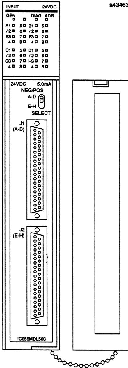
Figure 2-22. Typical I/O Module with Connectors
