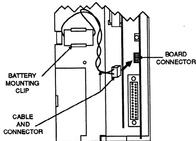
Figure 2-7. Back-Up Battery For CPU Functions
