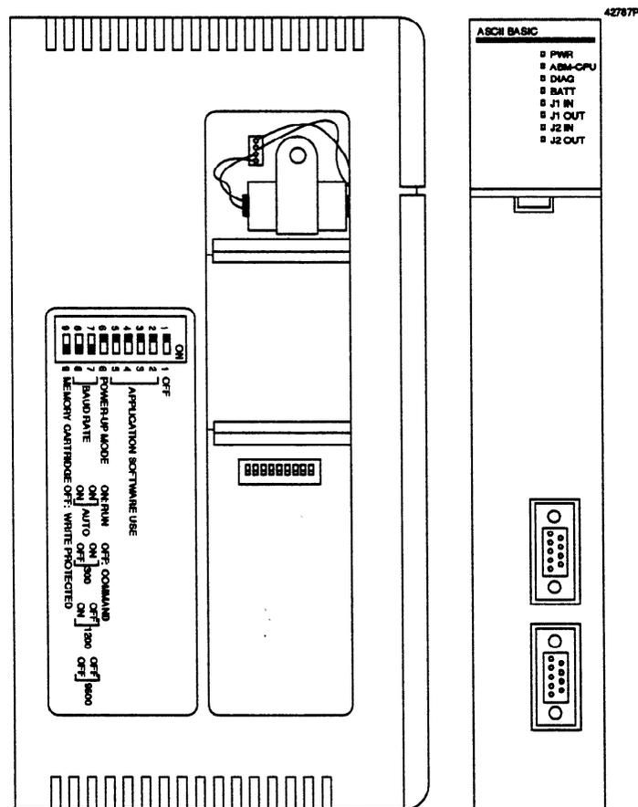
Figure 2-26. Series Five PLC ASCII/BASIC Module
