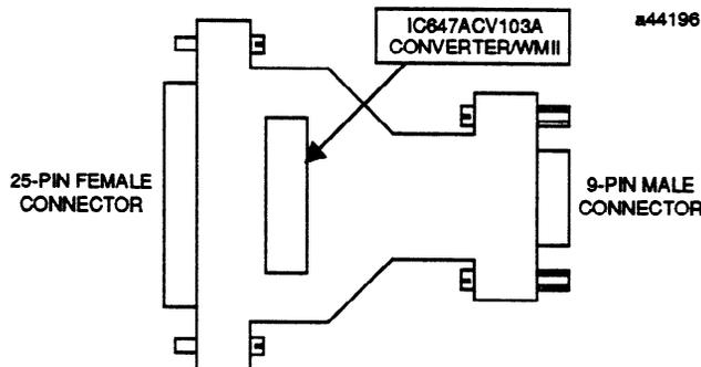
Figure 2-29. Connector Converter Assembly
