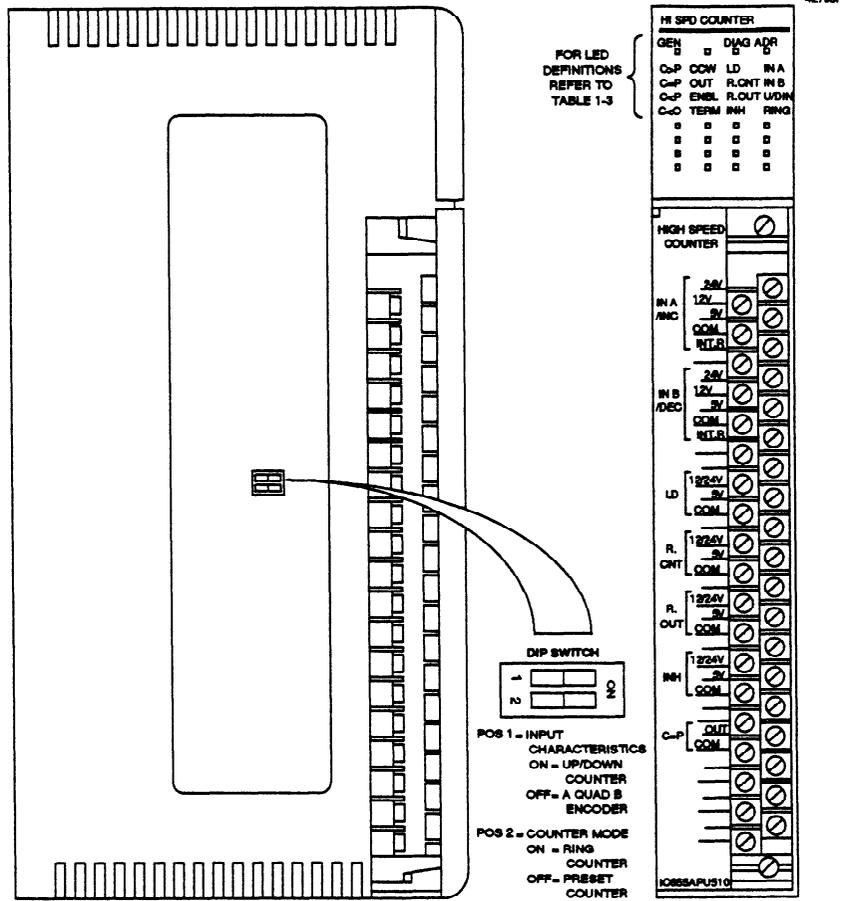
Figure 2-28. High Speed Counter Features
