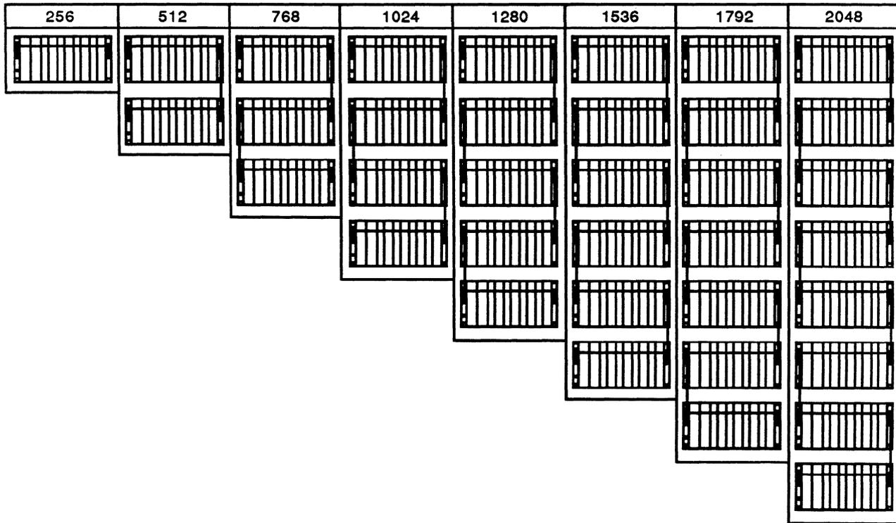
**Figure 2-16. Maximum I/O Contained in 1 to 8 Base Units**
