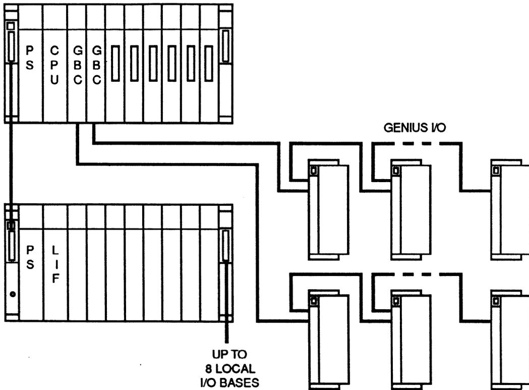
Figure 1-4. Example of Local I/O and Genius I/O System Configuration
