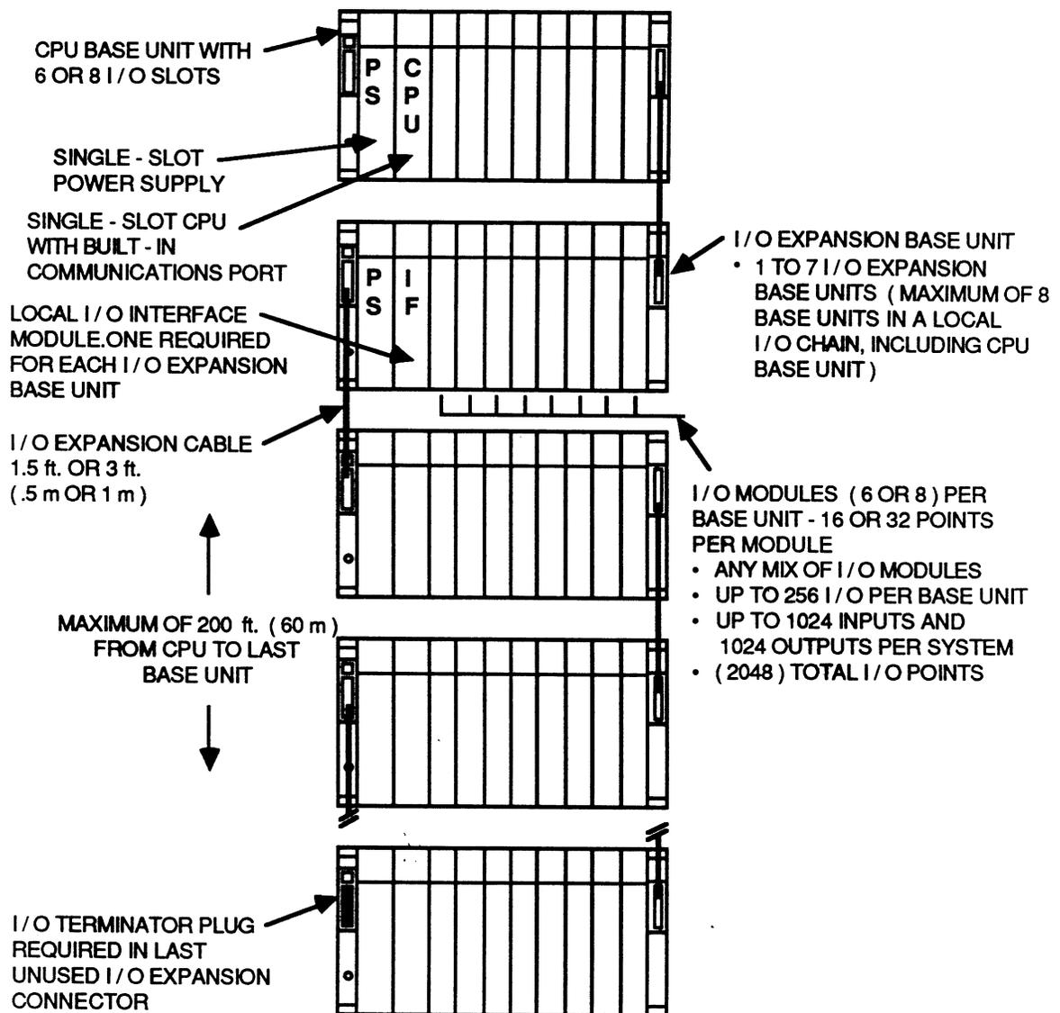
**Figure 1-3. Example of Series Five PLC Local I/O System Configuration**
