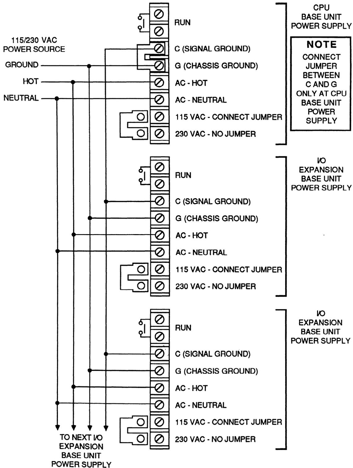
Figure 3-12. Example of Connecting Power Wiring to Multiple Base Units
