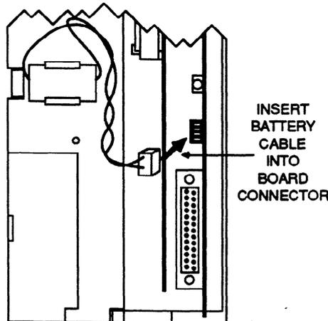
Figure 3-13. Back-Up Battery Mounting and Connection
