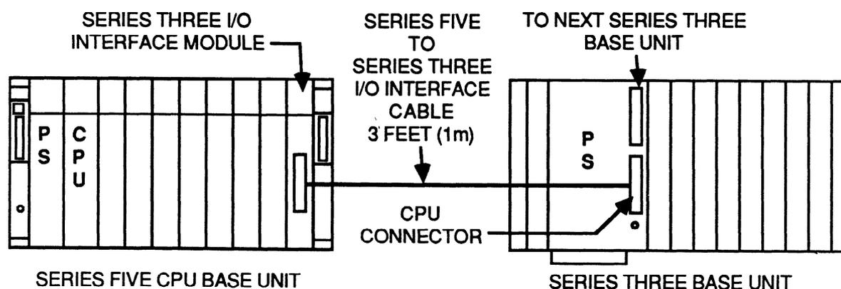
Figure 3-19. Series Three PLC I/O Interface to a Series Five PLC
