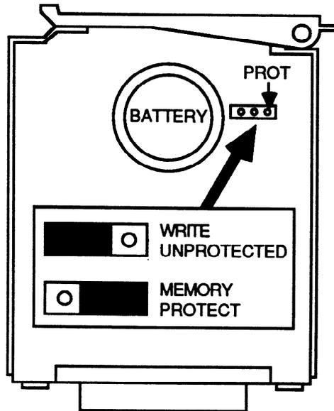
Figure 2-9. Memory Protect Configuration
