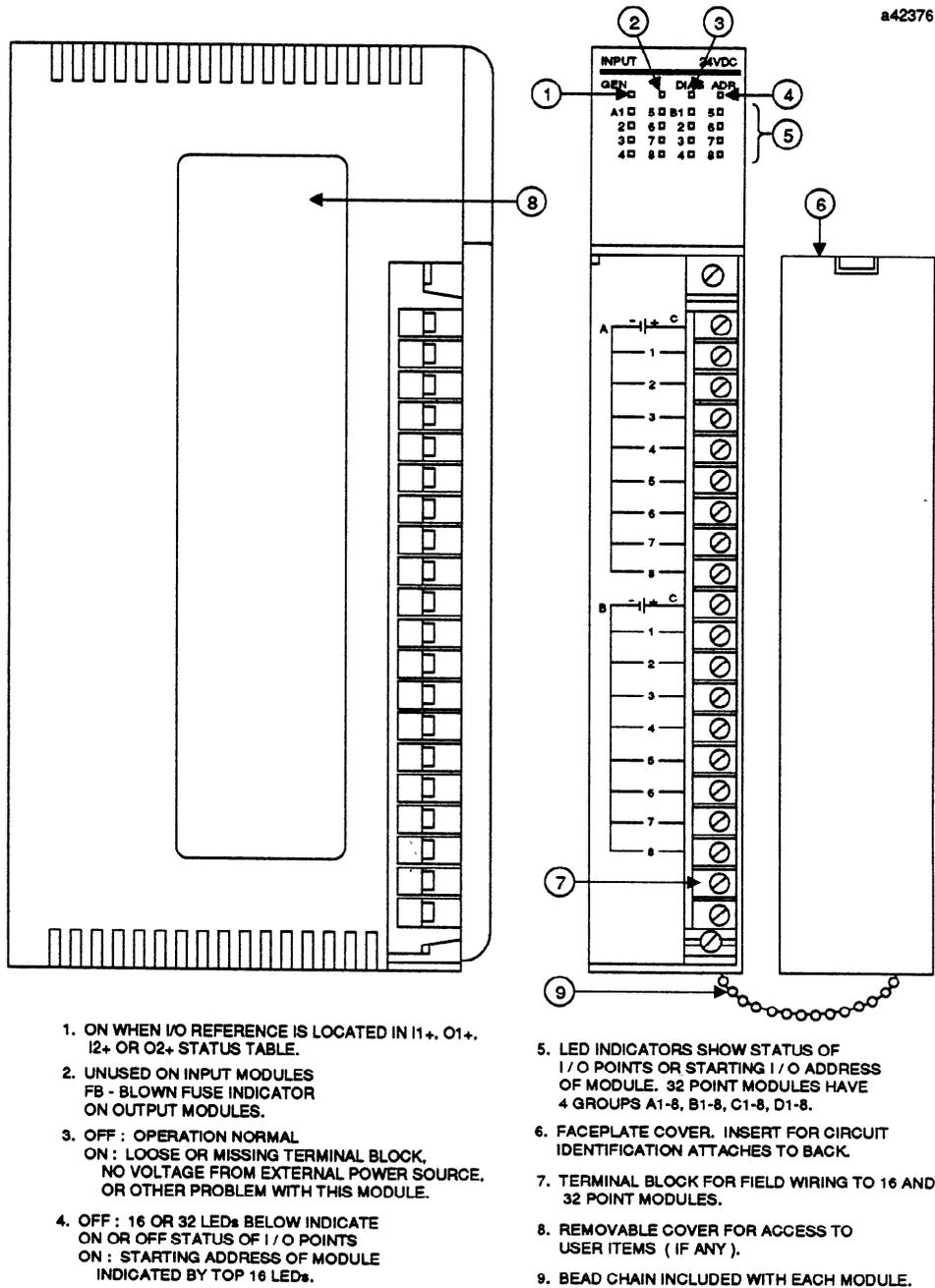
Figure 2-21. Typical I/O Module with Removable Terminal Block
