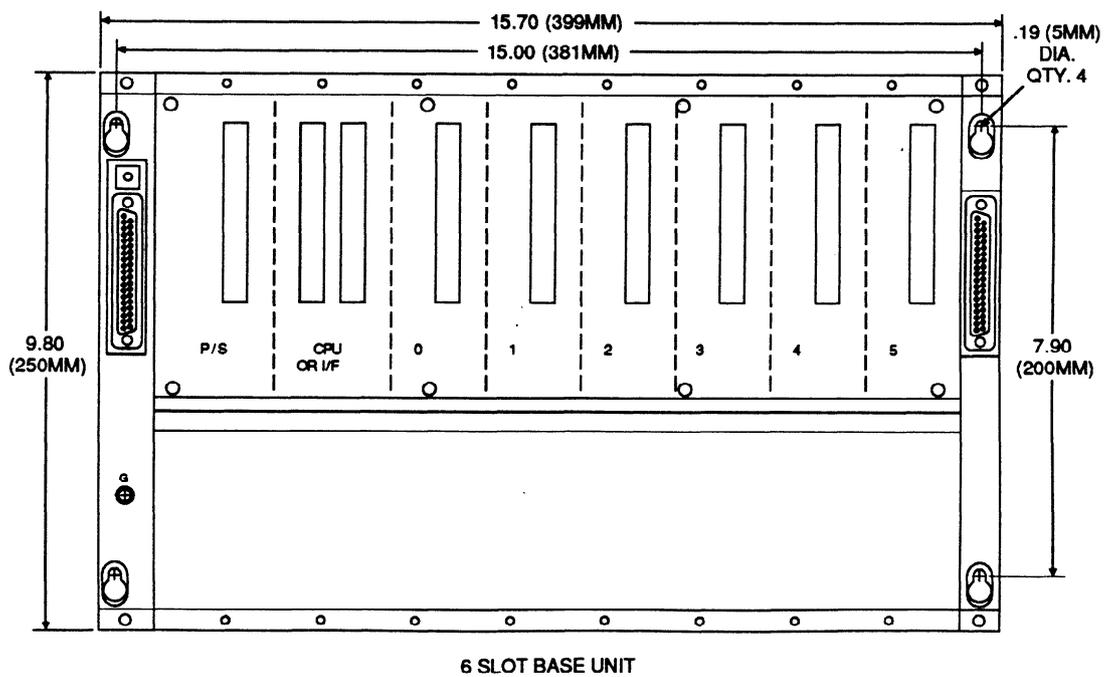
DIMENSIONS IN INCHES, MILLIMETERS ARE IN PARENTHESIS
