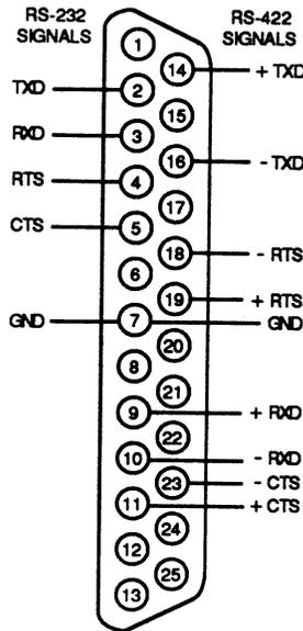
Figure 2-6. RS-232/RS-422 Communications Port Pin Assignments
