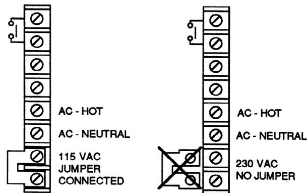
Figure 3-8. Terminal Jumper for AC Power Source Configuration.
