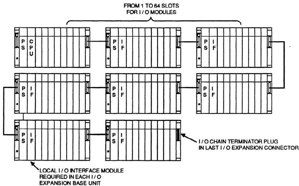
Figure 2-14. Example of Local I/O Expansion Chain
