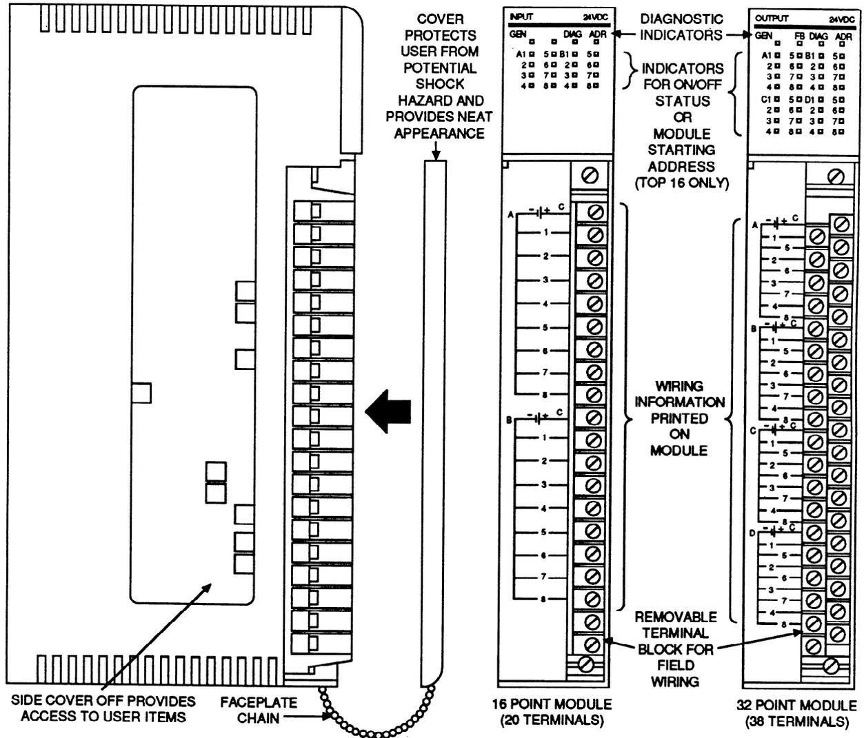
Figure 3-17. Typical I/O Module
