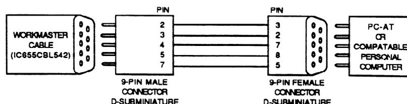
Figure 2-31. Cable for Series Five PLC to PC-AT Computer
