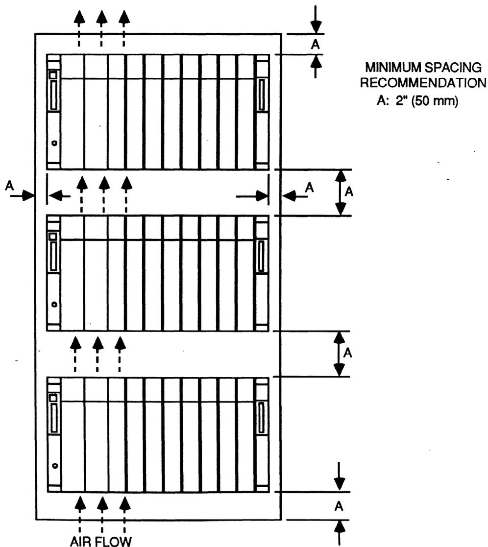
Figure 2-15. Base Unit Mounting for Proper Heat Dissipation
