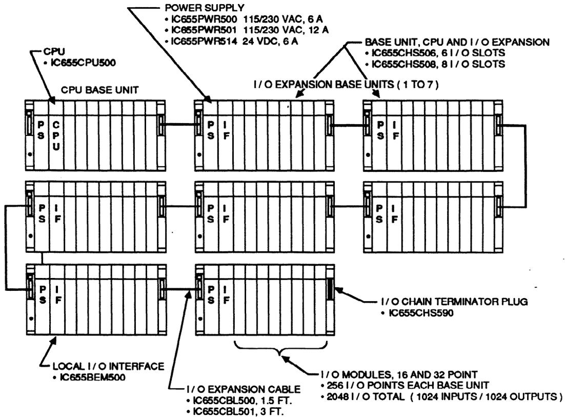
Figure 3-3. Connection of I/O Expansion Base Units
