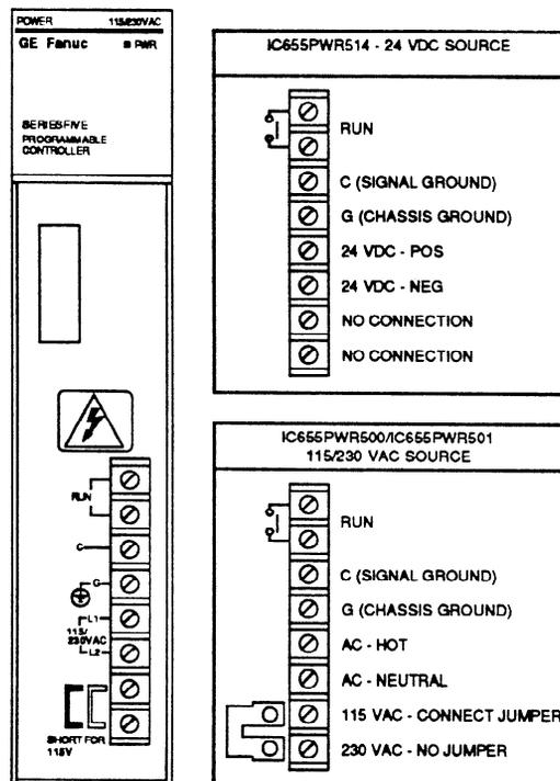
Figure 2-12. Power Supply Terminal Block Connections
