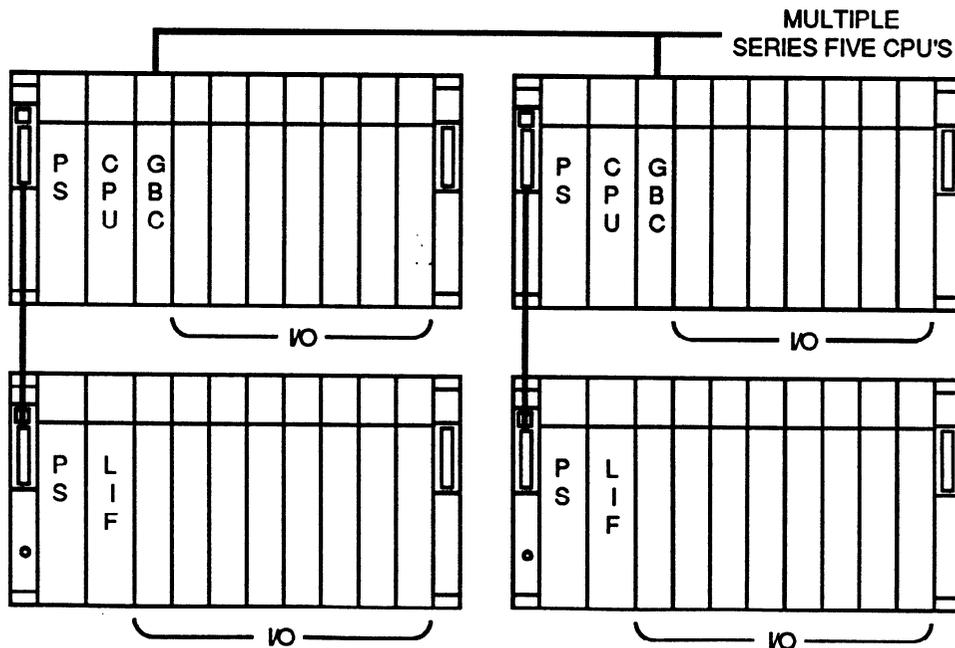
Figure 1-5. CPU-TO-CPU Communications Through GENIUS LAN
