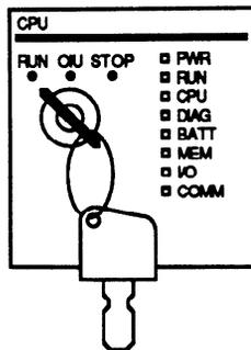
Figure 2-4. CPU Mode Switch
