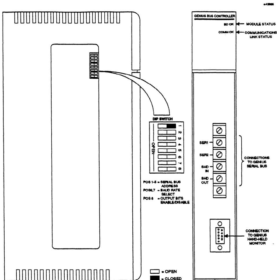
**Figure 2-24. Genius Bus Controller for the Series Five PLC**
