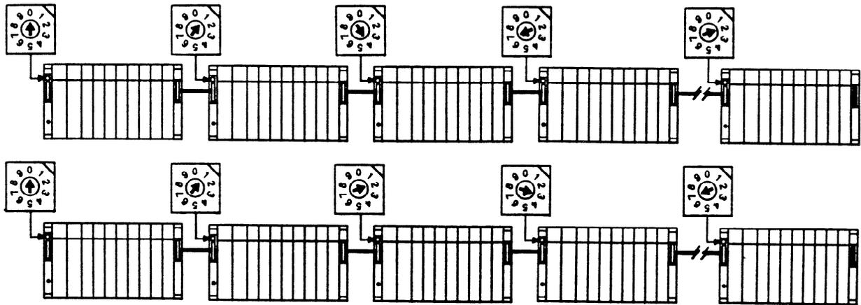
Figure 2-17. Examples of Base Unit Identification Switch Settings
