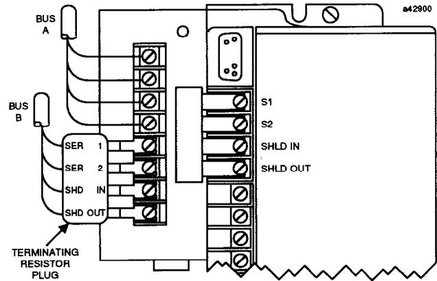
If both cables terminate at the BSM, install two resistors.
