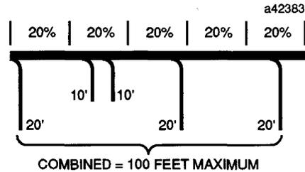
The locations of BSMs depend on the type of bus trunk cable and baud rate, as explained below.
