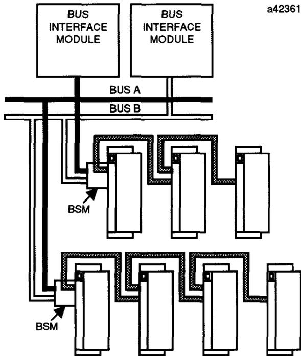
*This could be two 10' stubs with up to 8 blocks on each, or four 5' stubs, with fewer blocks on each. Additional BSMs can be located elsewhere on the bus.*
