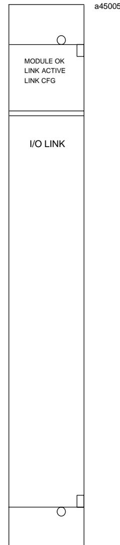
The I/O Link Module is configured using the MS-DOS® programming software. Application software, supplied on diskettes with the I/O Link Module, can be used to set up and control the I/O Link. This application software can also be used to assign the location of the input and output data to and from the I/O Link, and to provide diagnostics capabilities for the I/O Link. The MS-DOS programmer is used to integrate this application software with the rest of an application program.
